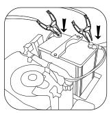
c. At this time, the green light on the main interface will flash, and the voltage of the Jumpstarter in parallel with the car battery will be displayed. After entering the start mode, if you want to only check the voltage of the car battery, short press the "Power" button to exit the start mode, the Jumpstarter will enter the measurement mode, and then the "green light" will go out, and the display only shows the voltage value of the car battery.
