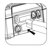
b. Connect the positive and negative of the clamps to the positive and negative of the car battery respectively, and make sure the connection is good;
